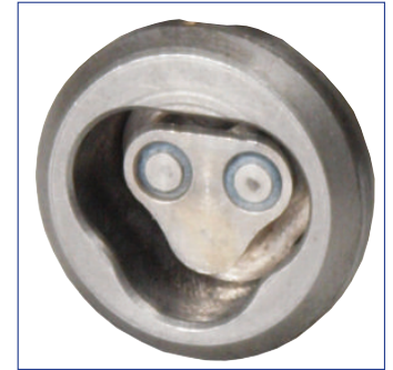
Figure 1 – Dirty Lock Face
